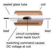
The input selectors on the MA6900 actually control stateof-the-art silent electromagnetic switches.
